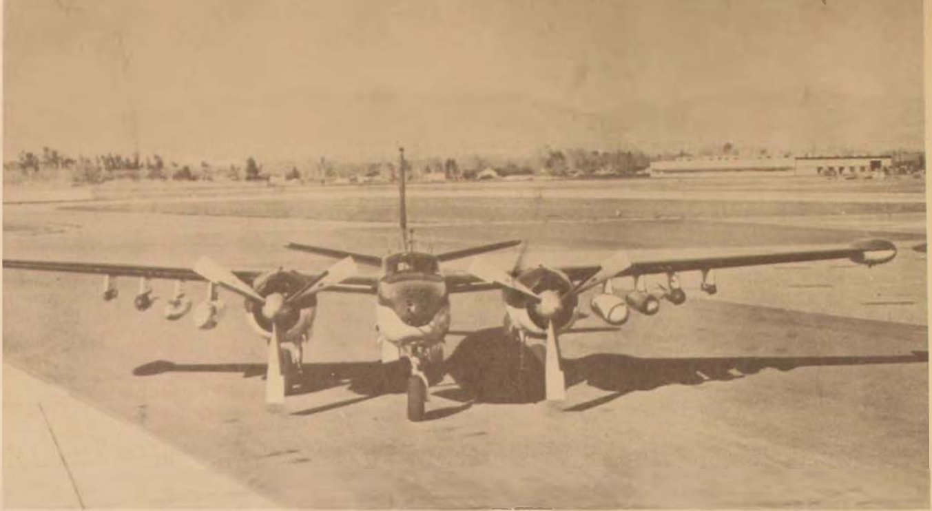
Loaded for combat. The new YB-26K or Counter Invader is shown on a ramp at Hill Air Force Base, April 1963. With rockets under its wings, eight aerial machine guns in its nose, and other features which add to its firepower and maneuverability, the Counter Invader is proving an invaluable asset in the Viet Nam Air Force for COIN missions.
