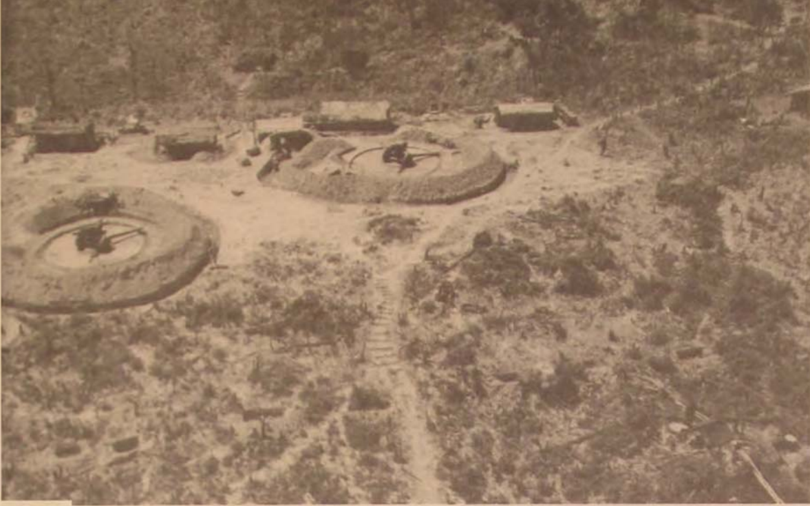
Point defense position of a remote Vietnamese post. Artillery weapons in circular revetments have 360° field of fire against ground attack.
